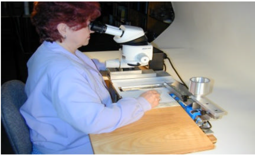
Fig. 2. The Ergovision Inspection Station is designed to reduce analyst's fatigue and discomfort.
